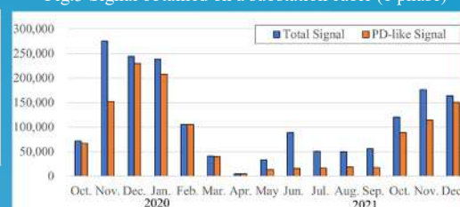
Fig.3 Signal obtained on a substation cable (1 phase)
